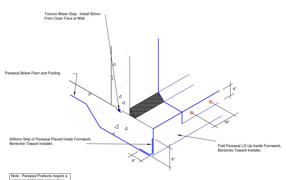
Note: Paraseal Products require a minimum 117 kg/m² compaction/ confinement to be effective.
