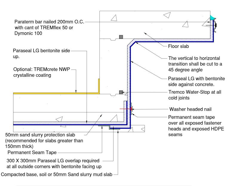
NOTE: Paraseal products require a min of 117kg/m2 of compaction/confinement in order to function as designed.
