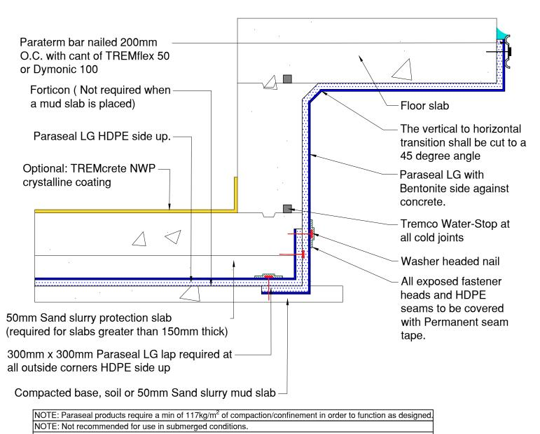
NOTE: If Mud Slab is not placed refrain from using chipped aggregate.
