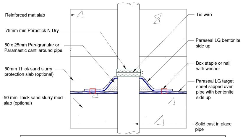
NOTE: Paraseal products require a min of 117 kg/m2 of compaction/confinement in order to function as designed.
