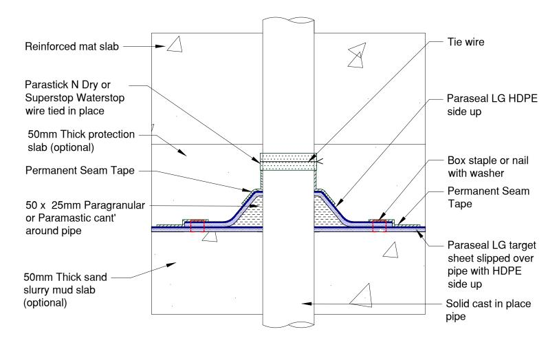
NOTE: Paraseal products require a min of 117kg/m2 of compaction/confinement in order to function as designed.
