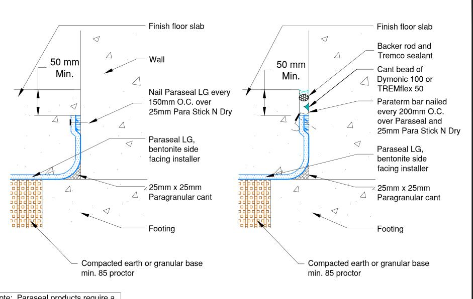
Note: Paraseal products require a minimum 117kg/m<sup>2</sup> compaction/ confinement to be effective.
