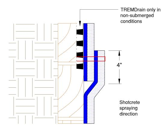
When spraying shotcrete or other materials against Paraseal LG, spray either directly at the seam or at the closed edge of the seam so as not to lodge sprayed materials between the lapped sheets. Never spray into open edge of seam.
