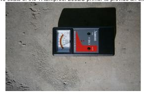
Pictured moisture reading of a Concrete Screed
